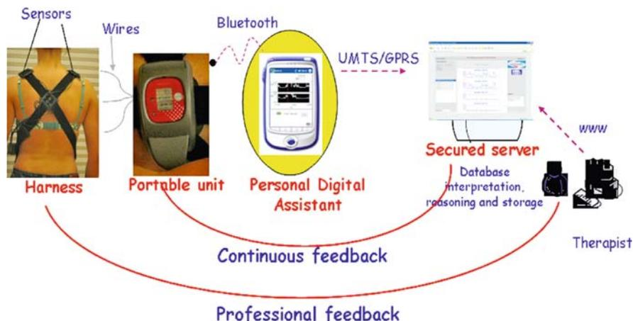
**Fig. 36.2** Components, data transmission, and ways of feedback provision in the MYOTEL intervention.
